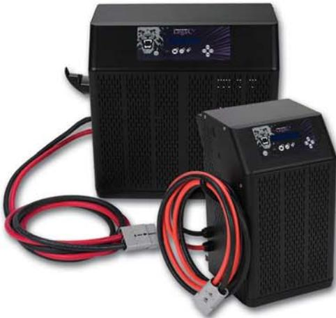
To maintain peak efficiency at all times, Legac<sup>2</sup> chargers are designed to switch power modules on and off automatically. If a single module develops a minor fault, Legac<sup>2</sup> chargers will simply bypass it and continue operating at reduced power. The charging process will continue uninterrupted, along with your fleet operations.
